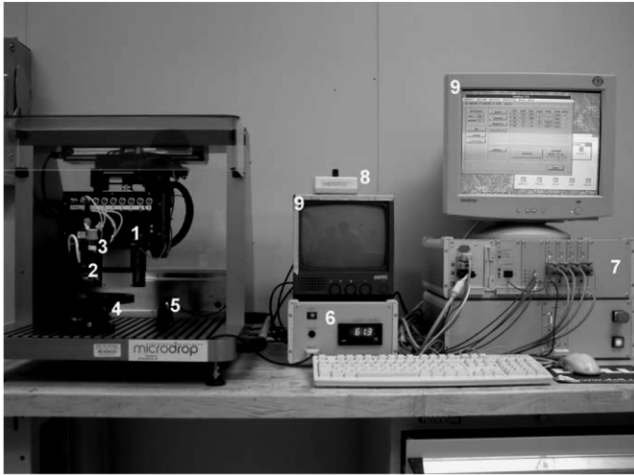
Fig. 1. Autodrop dispensing system with dispensing heads from Microdrop GmbH in Germany (1: x - y - z positing system; 2: camera 1; 3: solution reservoir; 4: substrate holder/hotplate; 5: camera 2; 6: temperature control system; 7: Driver electronics/pressure control; 8: Camera switch; 9: Monitor).
