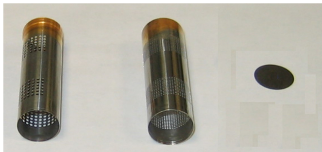
Fig. 8. Mechanical components including the anode support (left), cathode electrode (center) and the anode electrode (right). The top of the anode support and cathode electrode are electroplated with gold to reduce contact resistance.
